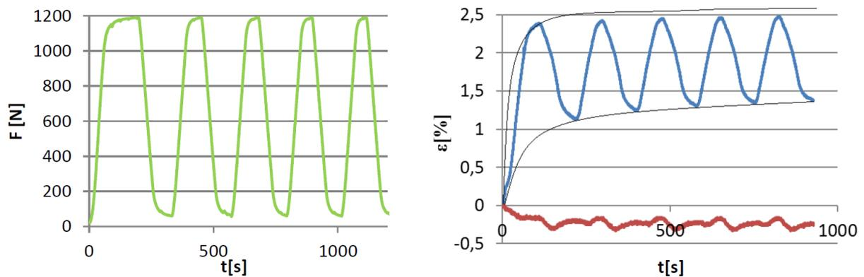
Figure 4: Stimulus and response functions recorded during cyclic biaxial test performed on white PVC membrane of  $900 \text{ g/m}^2$  area density
