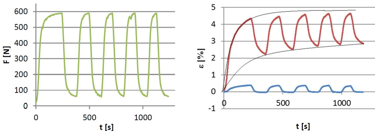
Figure 6: Stimulus and response functions recorded during cyclic biaxial test performed on yellow PVC membrane of  $350 \text{ g/m}^2$  area density
