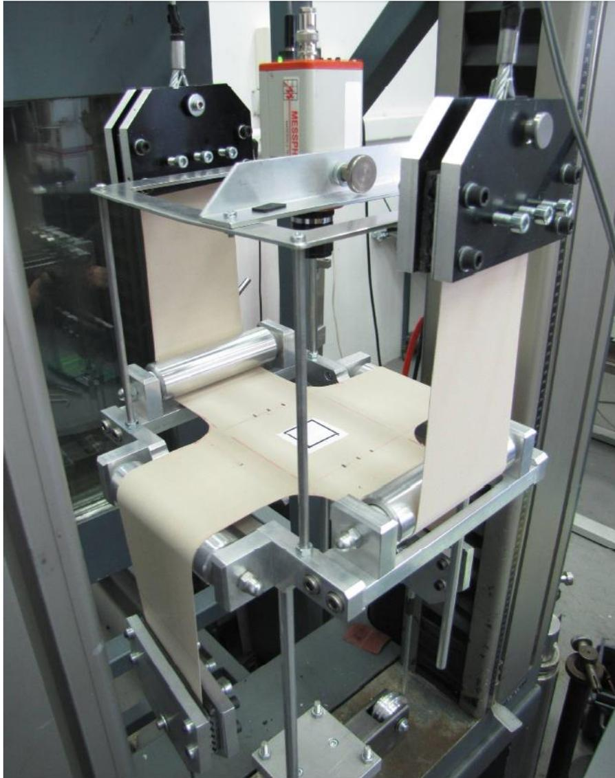
Figure 3: The elaborated biaxial testing apparatus for cyclic biaxial tests
