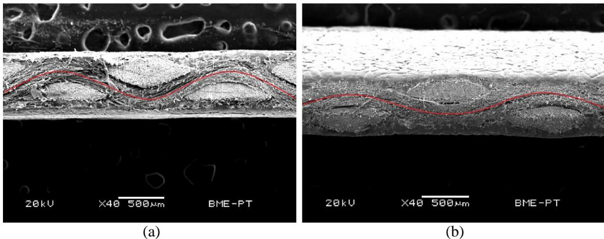
Figure 9: Cross section of the PTFE/GF technical textile specimen from the warp direction (a) and from the weft direction (b)
