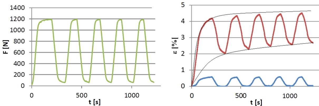
Figure 5: Stimulus and response functions recorded during cyclic biaxial test performed on grey PVC membrane of  $630 \text{ g/m}^2$  area density
