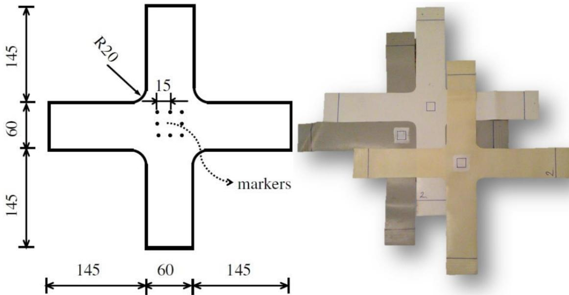
Figure 2: Standard cross-shaped textile samples for biaxial test
