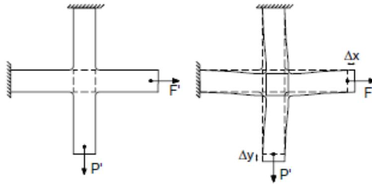
Figure 1: Displacement of the center of sample in case of equipment with two actuators [4]
