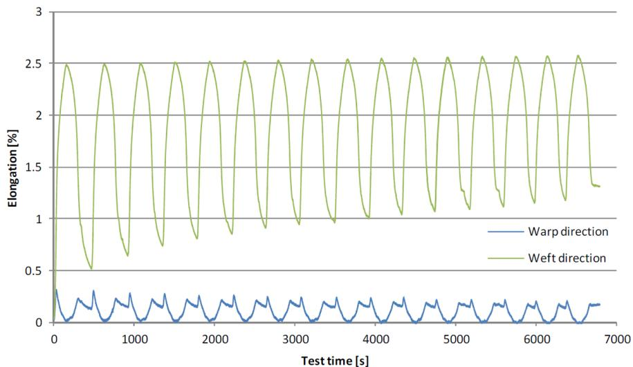
Figure 8: Registered elongation-time diagrams of the cyclic biaxial test at the PTFE/GF technical textile samples
