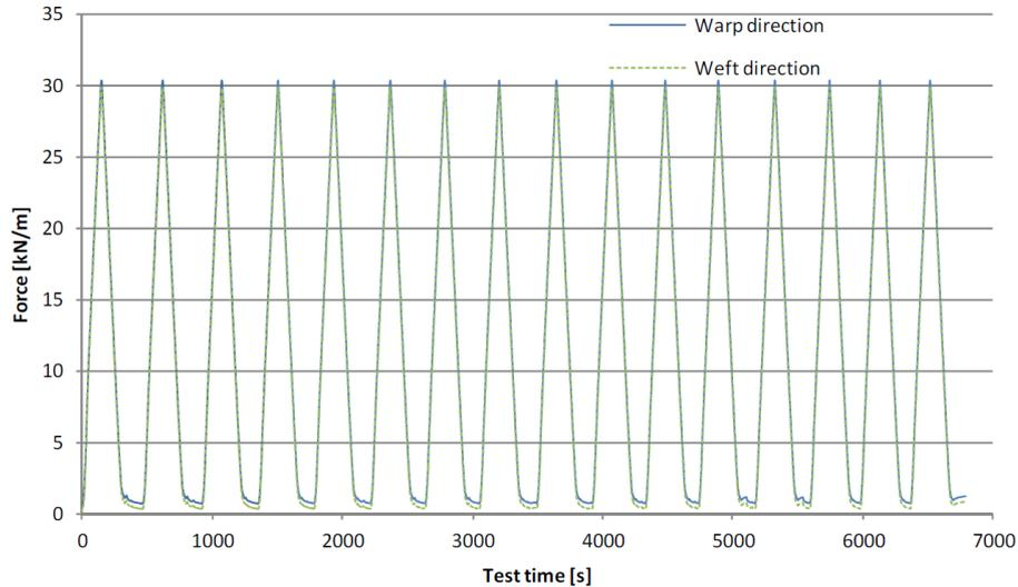
Figure 7: Registered force-time diagrams of the cyclic biaxial test at the PTFE/GF technical textile samples
